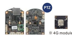
FS-I55F(T31N+GC4053):Fixed lens FS-I75E(T31X+GC4023):MFZ lens
